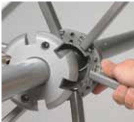
HUB The hub is cast aluminum and engineered for extra strength. It is split horizontally to encapsulate the stainless steel direct connect pin assembly. Two screws secure the hub together.
